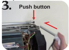
3.Push in "C shaped support bracket" of closed type cleaning cover to the hole on the plastic board, if inserted properly you will hear "Ka" sound.
